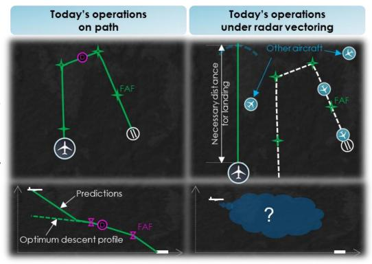
With current systems and practices, the crew must use rules of thumb and **subjective evaluation of remaining miles** to perform and monitor an efficient descent to the destination.
